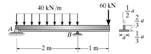
八、试求图示外伸梁截面 C 的挠度及截面 B 的转角,设 EI 为常数。[For the beam and loading shown, determine the deflection at section C and the slope at section B. EI is constant.](15 分)
