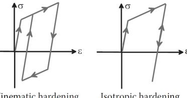
Kinematic hardening Isotropic hardening
