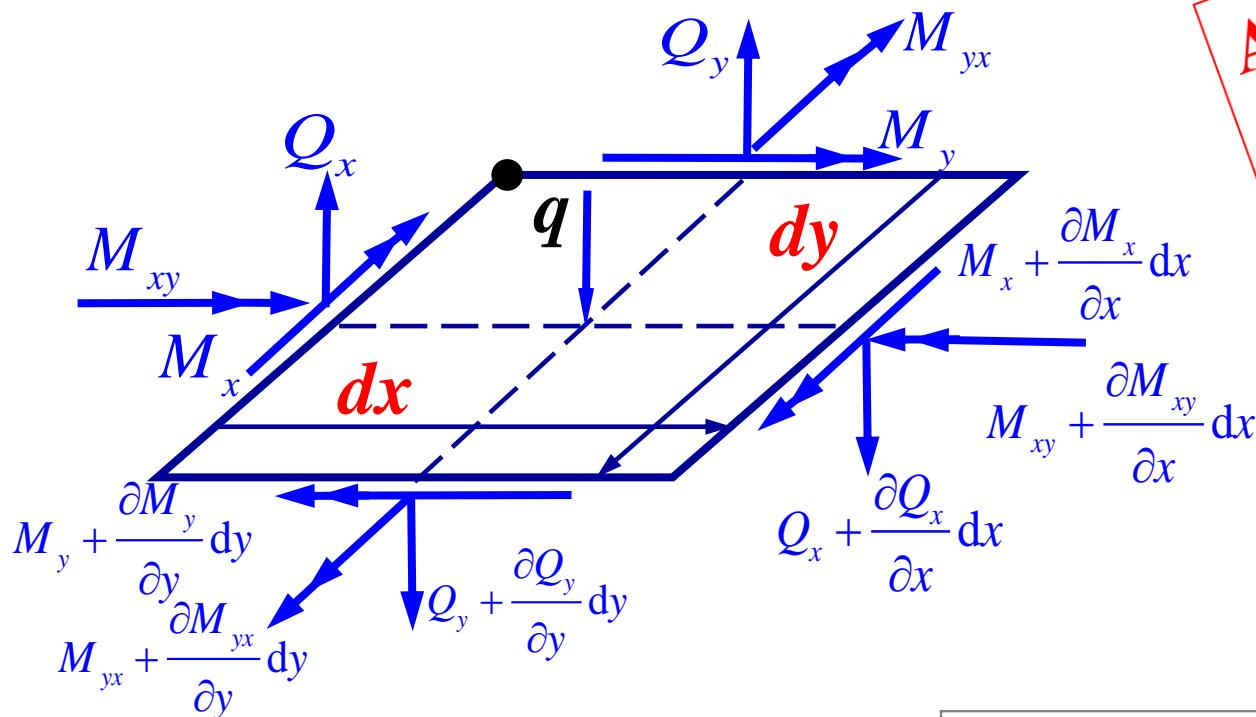
$$0 = \sum F_z = \frac{\partial Q_x}{\partial x} dx dy + \frac{\partial Q_y}{\partial y} dy dx + q dx dy \Rightarrow \boxed{\frac{\partial Q_x}{\partial x} + \frac{\partial Q_y}{\partial y} + q = 0}$$
