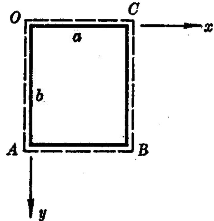
$$\boxed{\begin{aligned} (w)_{x=0} &= (w)_{x=a} = (w)_{y=0} = (w)_{y=b} = 0 \\ (M_x)_{x=0} &= (M_x)_{x=a} = (M_y)_{y=0} = (M_y)_{y=b} = 0 \end{aligned}}$$
