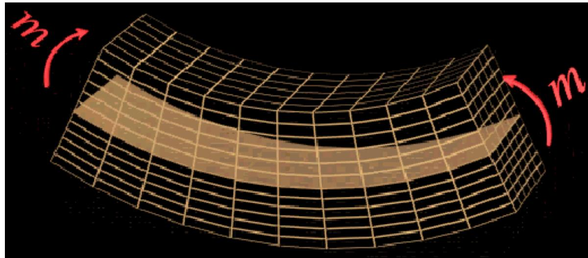
$$EI \frac{d^2 w}{dx^2} = M , \quad \frac{d^2}{dx^2} \left( EI \frac{d^2 w}{dx^2} \right) = q$$
