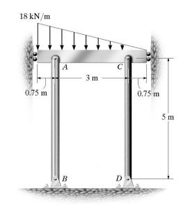
4. The steel bar *AB* has a rectangular cross section. If it is assumed to be pin connected at its ends, determine if member *AB* will buckle if the distributed load w = 2 kN/m. Use a factor of safety with respect to buckling of 1.5.  $E_{st} = 200$  GPa,  $\sigma_p = 194$  MPa.
